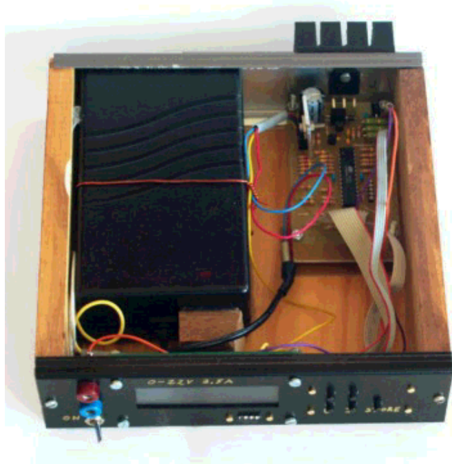
How it looks inside. I used an old 24V 3A laptop power supply "brick" as power source. They are very compact and don't need additional rectifiers or capacitors.
